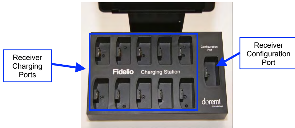
Figure 7: Fidelio Configuration/Charging Station - Top View
