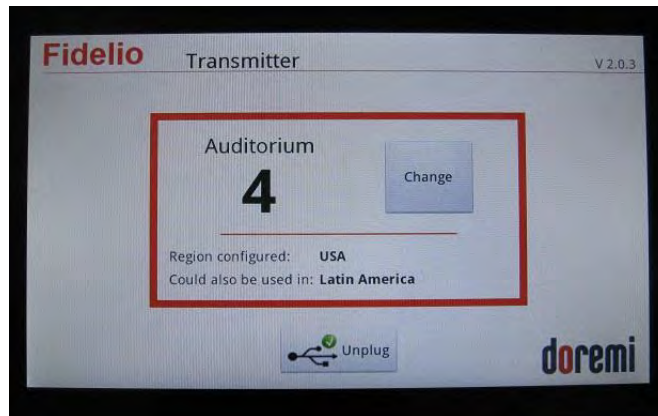
Figure 26: Transmitter Change Auditorium Screen
