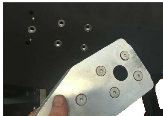
Place the screws included in the set in the spear, and mount them in the nuts.
