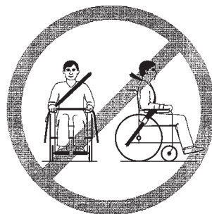
Incorrect use of belts
