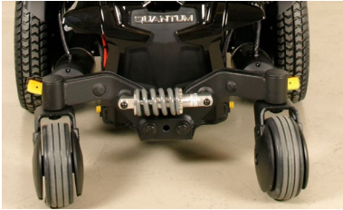
Normal position for driving - pushed up
