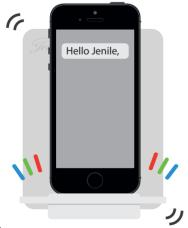
When you receive a call or a text message, the SMS Flasher lights up with multicoloured lights for one minute.
