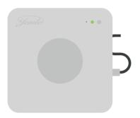
in green when the battery is charging. When the LED (F) is not lightened up, it means that it is operating normally.
