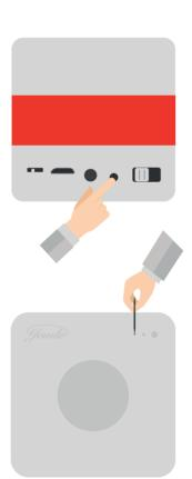
Press the plug button on your receiver (the cube, vibrator pocket, etc, ...)
