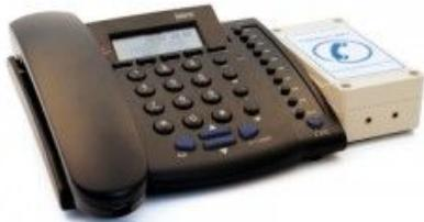
Enabler Phone allows you to **control a hands-free phone remotely** by using [our controllers](#) or locally using your favourite **switch**. You can make calls with the speed dial function or digit dialing, as well as answer and hang up in an autonomous way. Speak with whoever you want as much as you want!
